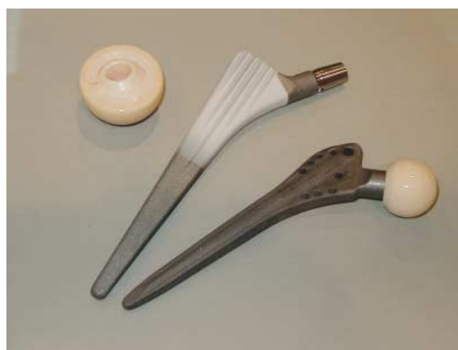
Figure 10. Calcium phosphates in hip endoprostheses: a ceramic ball joint ( \text{Al}_2\text{O}_3 ), a calcium-phosphate coated endoprosthesis (“cementless endoprosthesis”) and an uncoated endoprosthesis that must be fixed in place with PMMA bone cement.
